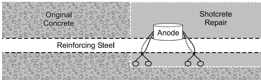
**Figure 1. Diagram of Anode and Placement**
