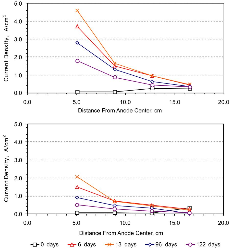
**Figure 18. Current Density Measurements at Sacrificial Anode Monitoring Devices in (top) Pier 1 and (bottom) Pier 12**
