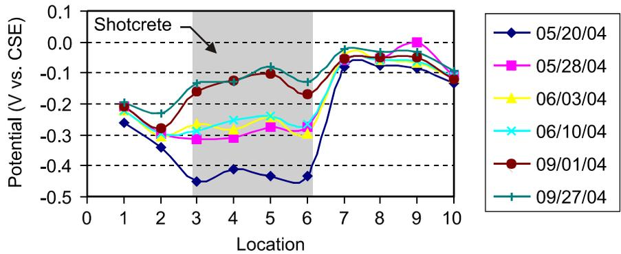
Figure 15. Half-Cell Measurements Versus Location for Column P12, Which Contains Sacrificial Anodes
