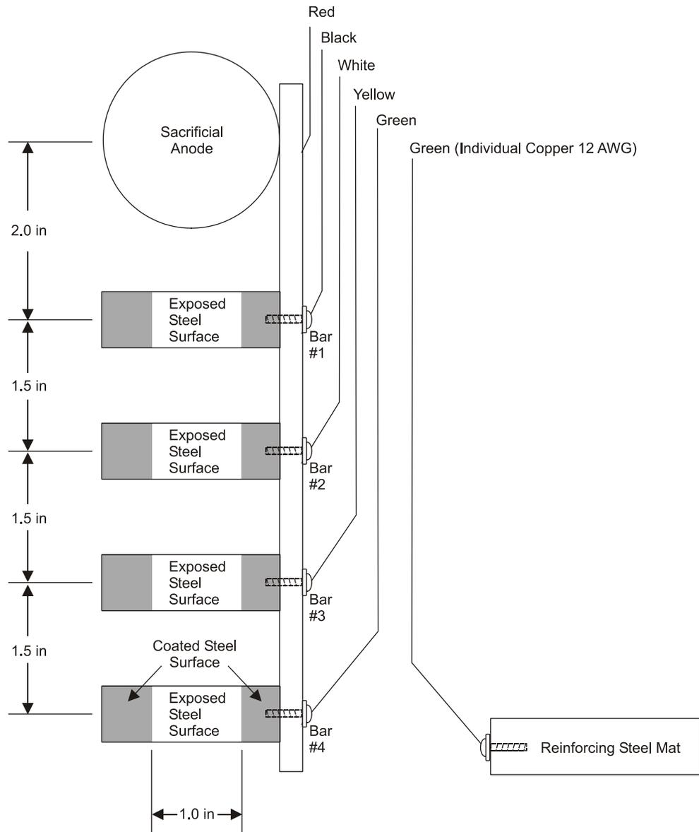
**Figure 7. Sacrificial Anode Monitoring Device**
