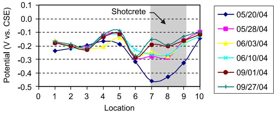
Figure 13. Half-Cell Measurements Versus Location for Column P1, Which Contains Sacrificial Anodes
