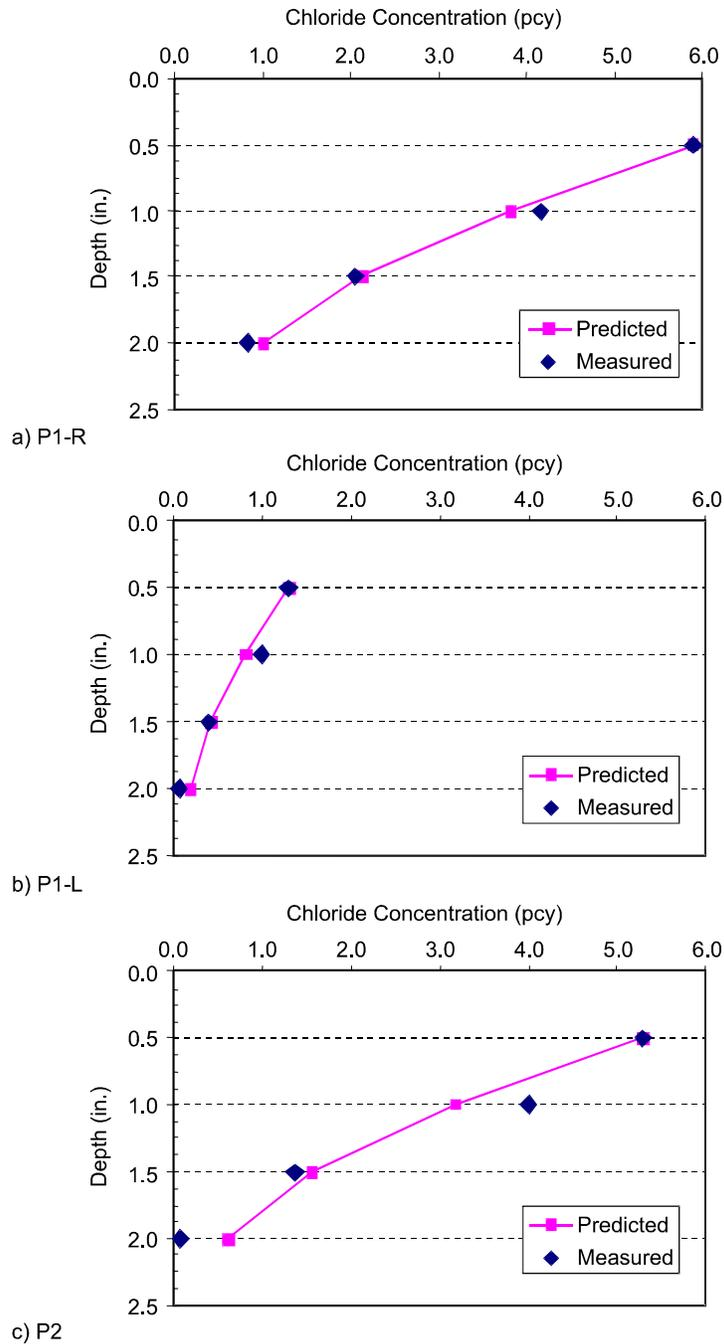
**Figure 11. Chloride Concentration Profiles Adjacent to Repairs at Location P1-R, P1-L, and P2**
