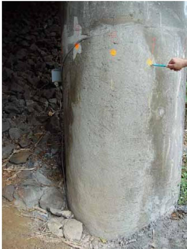
**Figure 4. Electrical Potential and Resistivity Test Locations After Repair**
