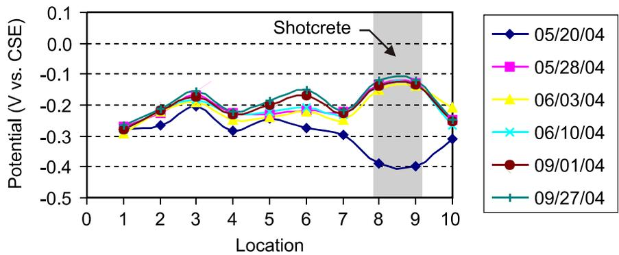
Figure 14. Half-Cell Measurements Versus Location for Column P2, Which Does Not Contain Sacrificial Anodes
