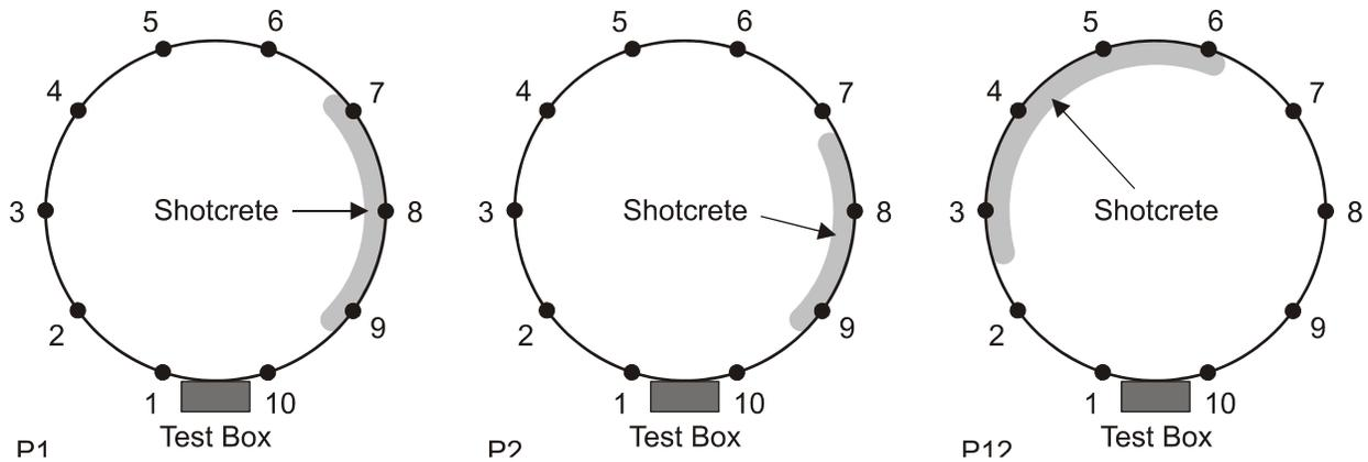
Figure 5. Electrical Test and Shotcrete Repair Locations on Each Column
