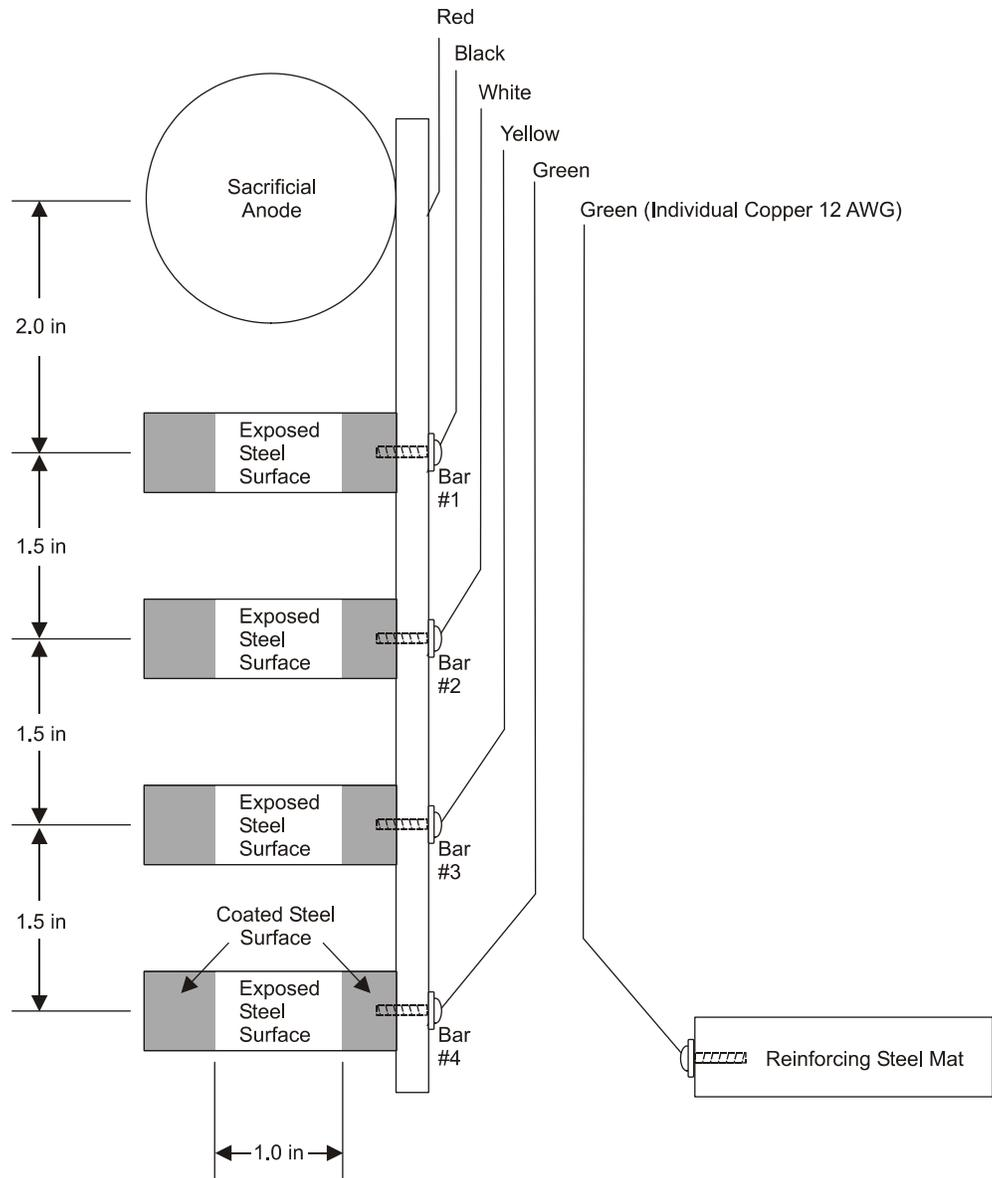
**Figure 7. Sacrificial Anode Monitoring Device**
