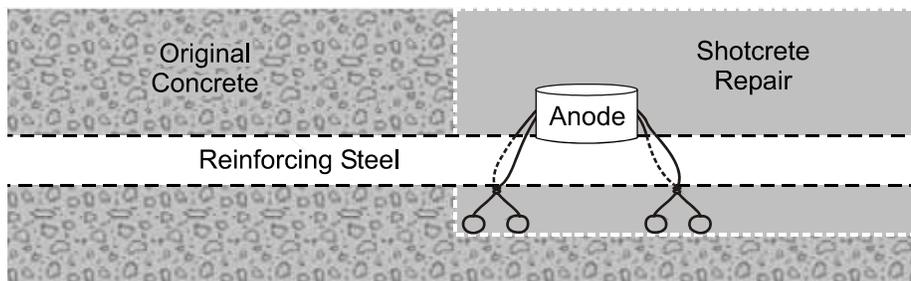
**Figure 1. Diagram of Anode and Placement**
