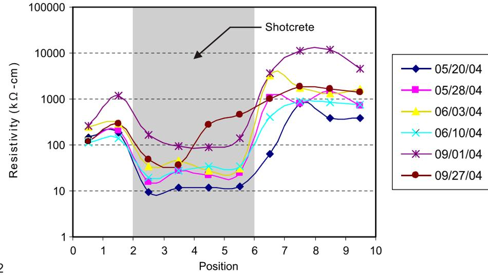
**Figure 16. Post-repair Resistivity of Concrete Versus Location**
