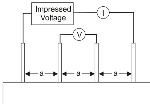
Figure 6. Four-Pin Resistivity Test Schematic
